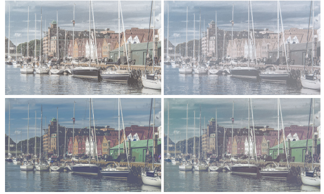
Fig. 14. Marked images on AISI 304 (top left) and AISI 430 (top right) with the same primaries explored and extracted on AISI 304. A newly explored and extracted set of primaries on AISI 430 are used for marking an image: gamut-mapped (bottom left) and photograph (bottom right). Image © Piotr Didyk.
