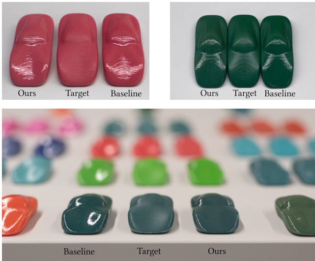
Figure 9: A small showcase of the color triads presented to test subjects during our experiment in different viewing angles and varnishes (top-left and bottom, Schmincke Matte , top-right, Edding Clear Matte ). Target denotes the target color appearance, while baseline is the same base color on the target surface finish. Ours achieves a closer perceived color to the target, while maintaining the desired glossy surface appearance. Note that due to compression and SDR screen quality, color differences may look substantially smaller than in real life.
