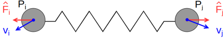
Figure 4. Spring damping force and velocities of the particles
