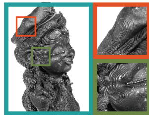
Figure 2: A 3D printed model with staircasing artifacts especially visible in the cheek and in the hat.
