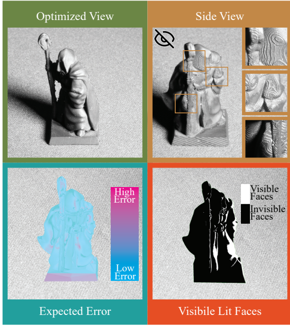
Figure 9: HOODED STRANGER model printed for Case 2 is shown in the figure. Our method excels at pushing artifacts to hidden areas. In this case left side of the model is in shadow, hence our method pushes artifacts onto this area. See that these errors are not visible from the optimized view point.
