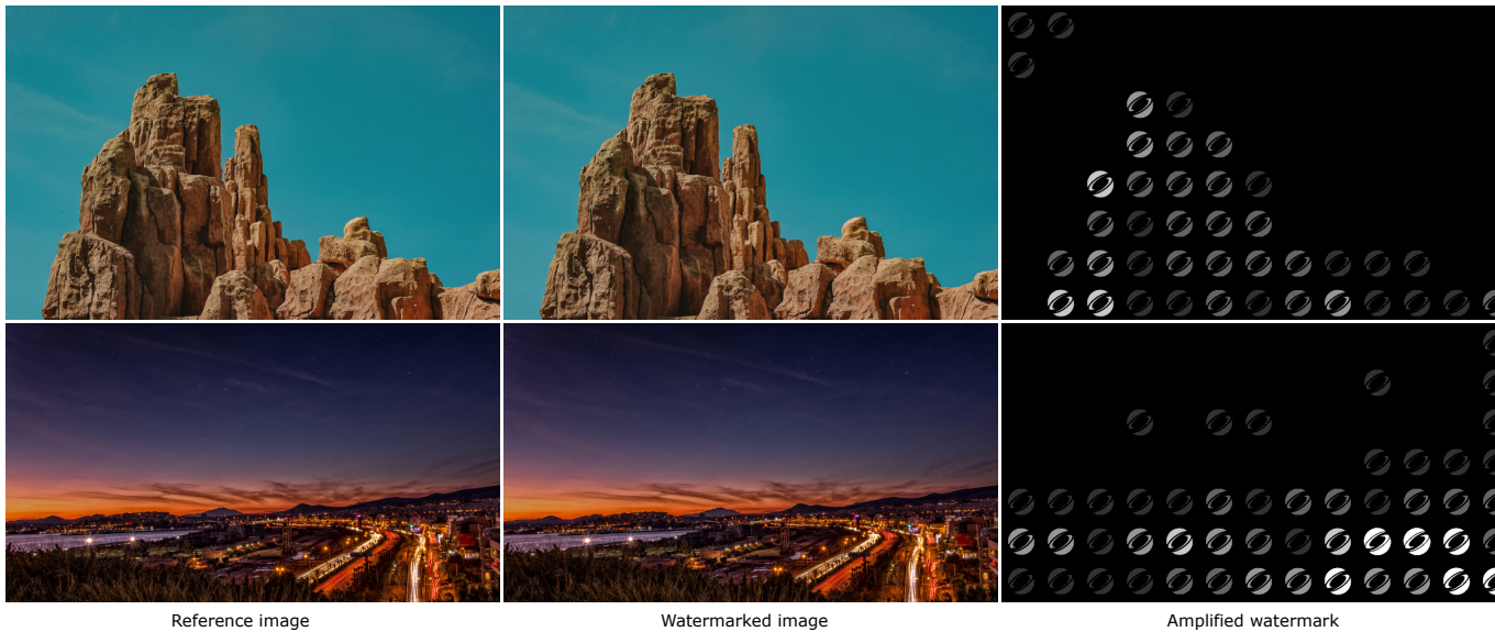
Fig. 14. Examples of content-adaptive watermark application. Our metric applies a brighter watermark in high frequency and contrast areas, like the rocks in the first example and city lights in the second example.
